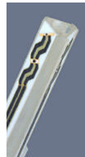
Figure 3.4 Probe Thick-Film Technique
