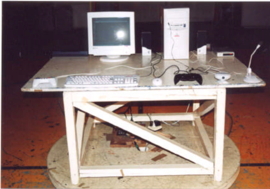
Photo 7.2a Setup with the Maximized RFI Field Strength Emission Level ( 30MHz ~ 1000MHz)
