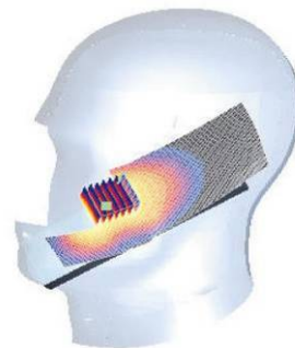
Figure 7-1 Sample SAR Area Scan
