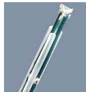
Figure 3.4 Probe Thick-Film Technique
