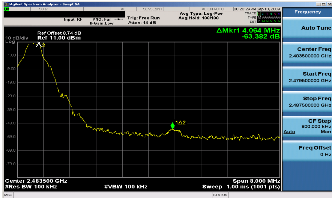
Plot 6-5. Band Edge Plot (Bluetooth – Ch. 78)
