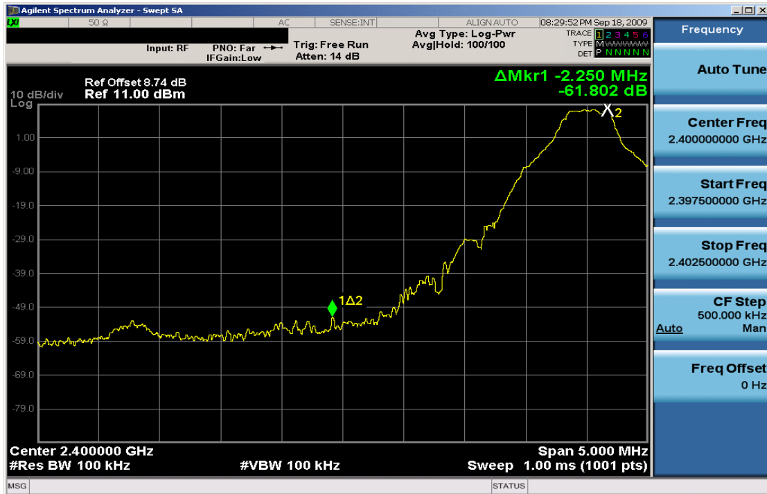
Plot 6-4. Band Edge Plot (Bluetooth – Ch. 0)
