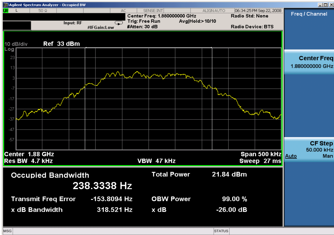
Plot 7-21. Occupied Bandwidth Plot (EDGE1900 Mode – Ch. 661)
