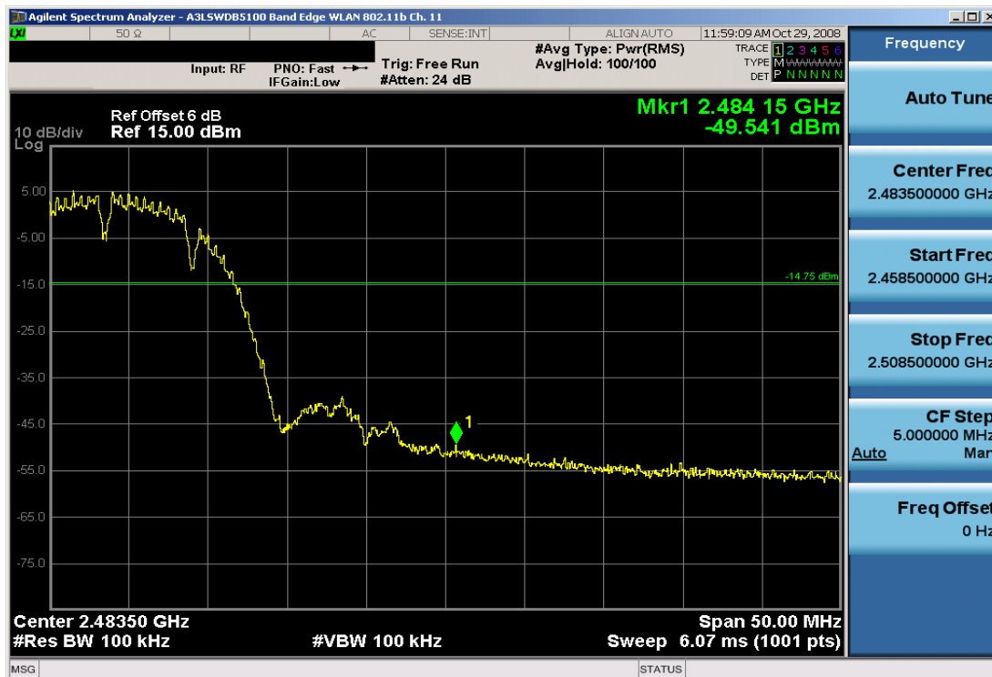
Plot 6-14. Band Edge Plot (802.11b – Ch. 11)
