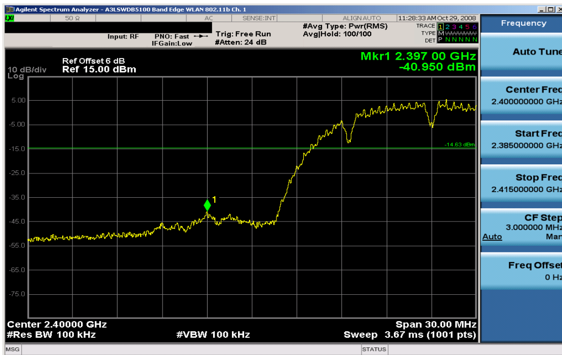
Plot 6-13. Band Edge Plot (802.11b – Ch. 1)
