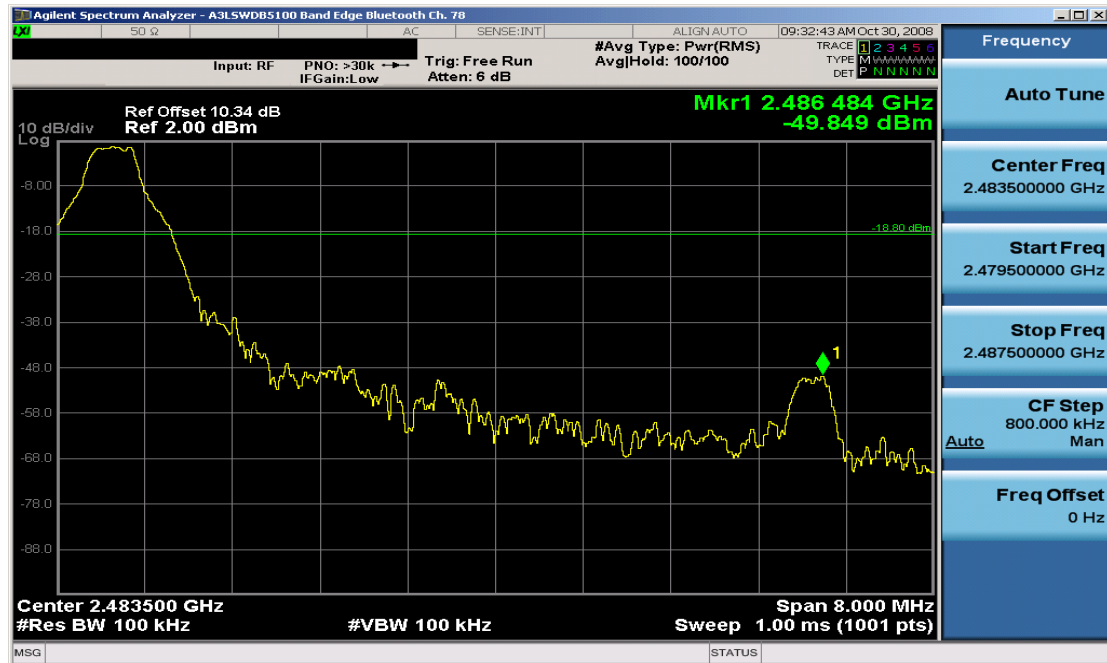
Plot 6-5. Band Edge Plot (Bluetooth – Ch. 78)
