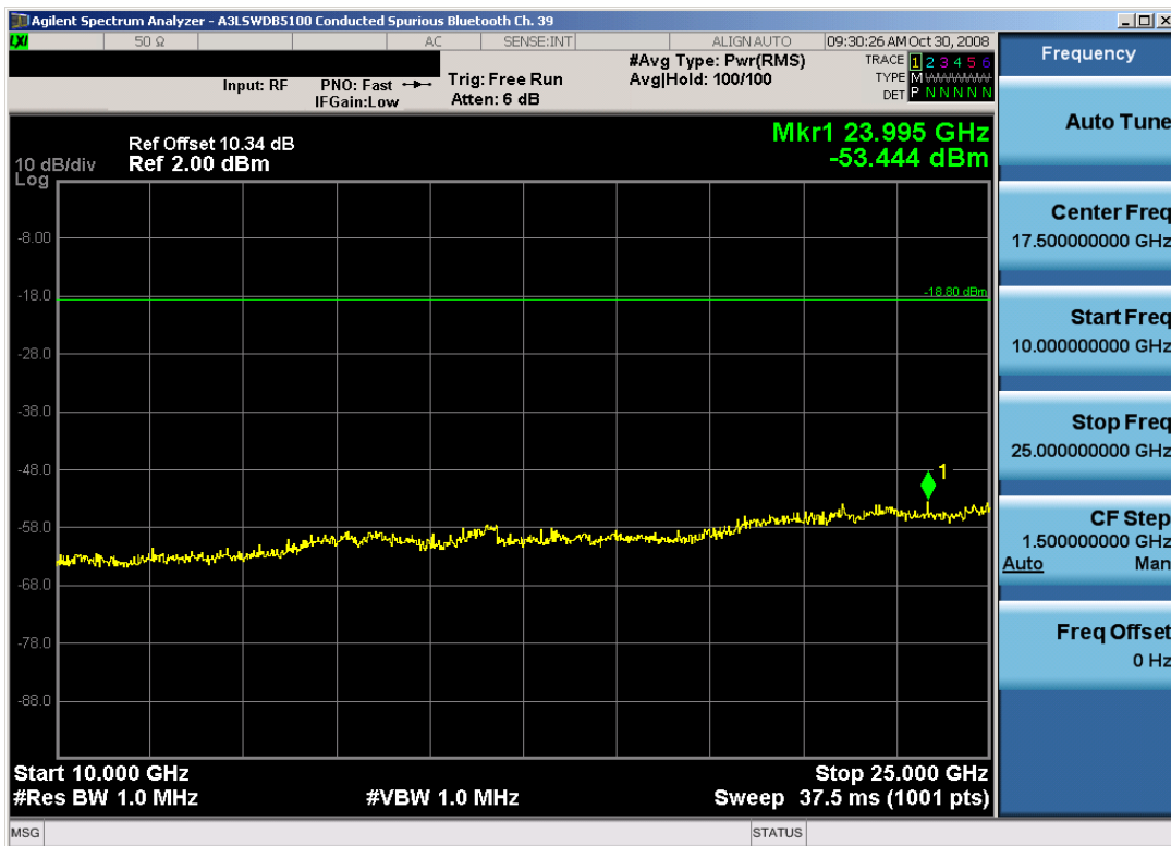
Plot 6-15. Conducted Spurious Plot (Bluetooth – Ch. 39)
