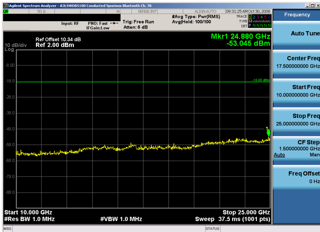
Plot 6-17. Conducted Spurious Plot (Bluetooth – Ch. 78)
