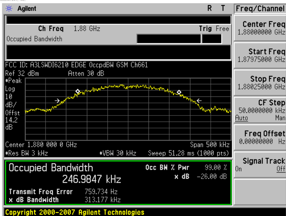
Plot 7-21. Occupied Bandwidth Plot (EDGE1900 Mode – Ch. 661)
