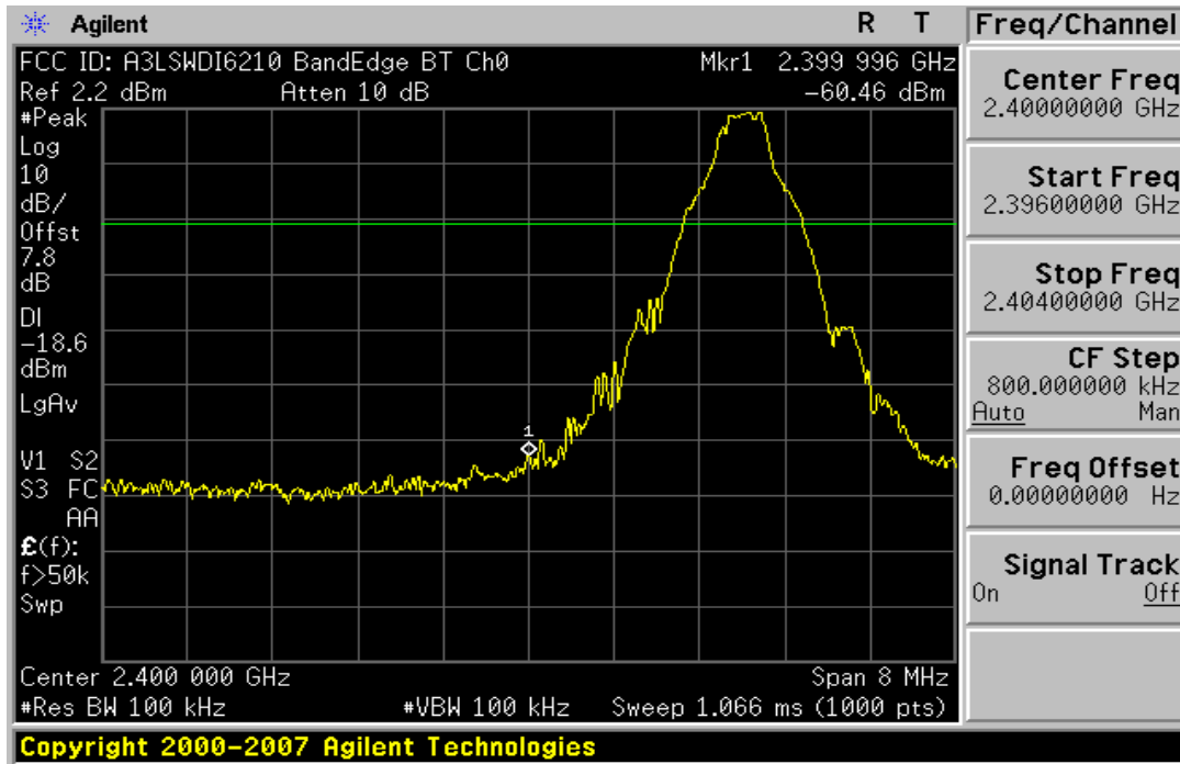
Plot 6-4. Band Edge Plot (Bluetooth – Ch. 0)
