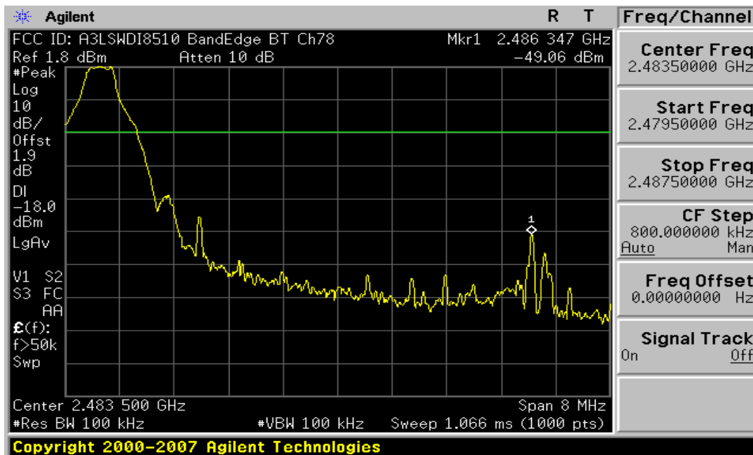
Plot 6-5. Band Edge Plot (Bluetooth – Ch. 78)
