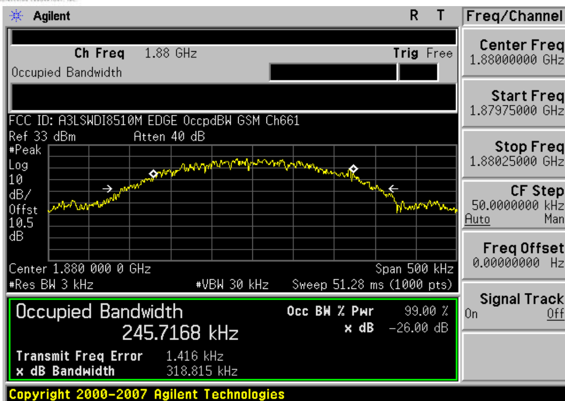
Plot 7-21. Occupied Bandwidth Plot (EDGE1900 Mode – Ch. 661)
