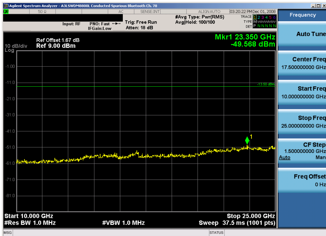
Plot 6-17. Conducted Spurious Plot (Bluetooth – Ch. 78)
