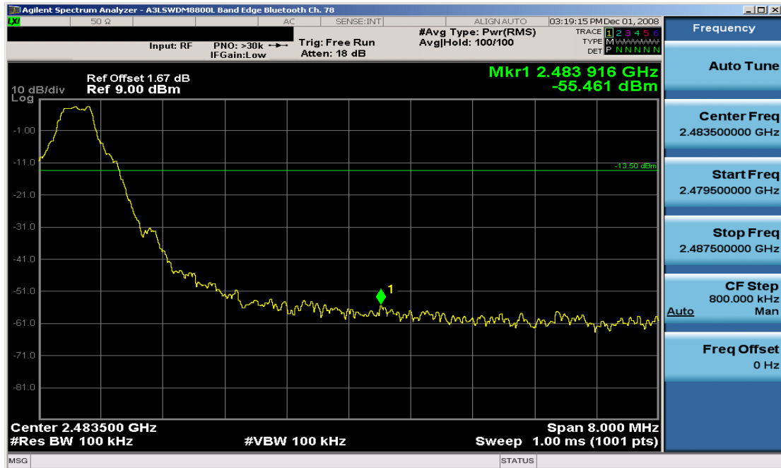
Plot 6-5. Band Edge Plot (Bluetooth – Ch. 78)
