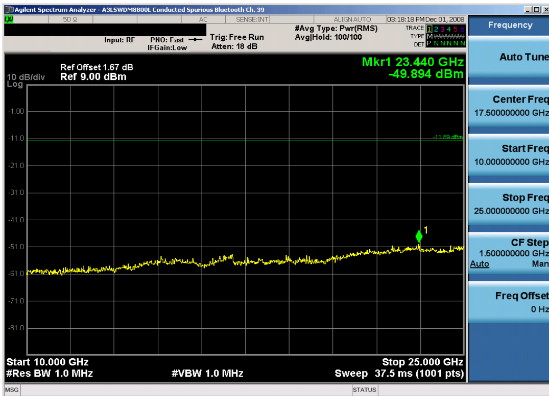
Plot 6-15. Conducted Spurious Plot (Bluetooth – Ch. 39)
