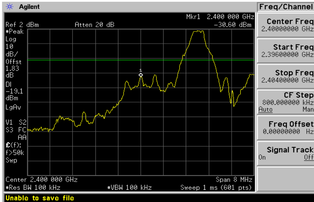
Plot 6-4. Band Edge Plot (Bluetooth – Ch. 0)
