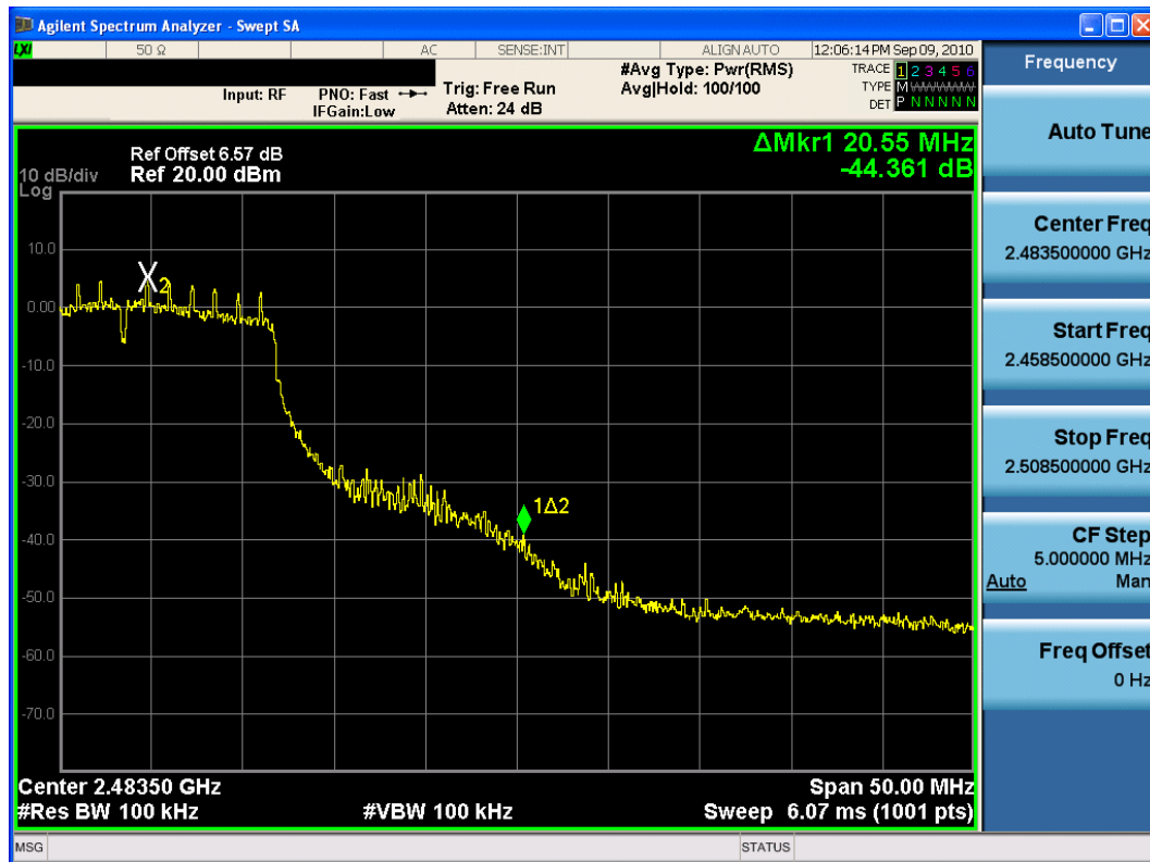
Plot 6-34. Band Edge Plot (802.11g – Ch. 11)
