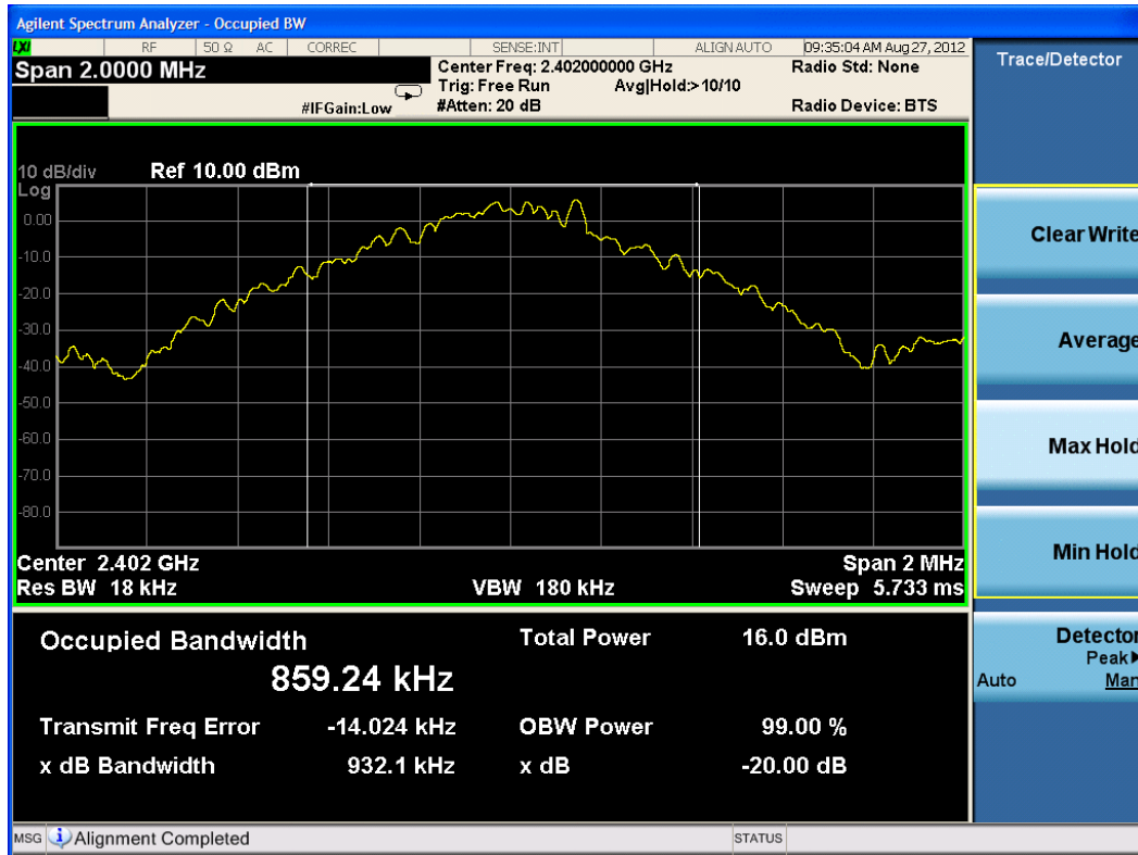
Plot 6-1. 20dB Bandwidth Plot (Bluetooth, 1Mbps – Ch. 0)
