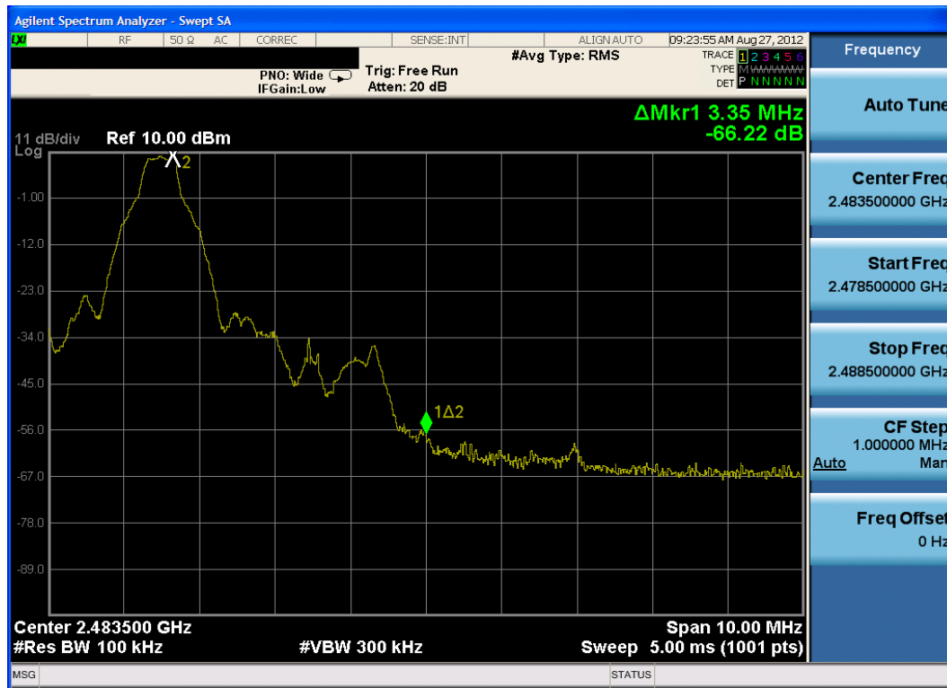
Plot 6-20. Band Edge Plot (Bluetooth with Hopping Disabled, 1Mbps – Ch. 78)
