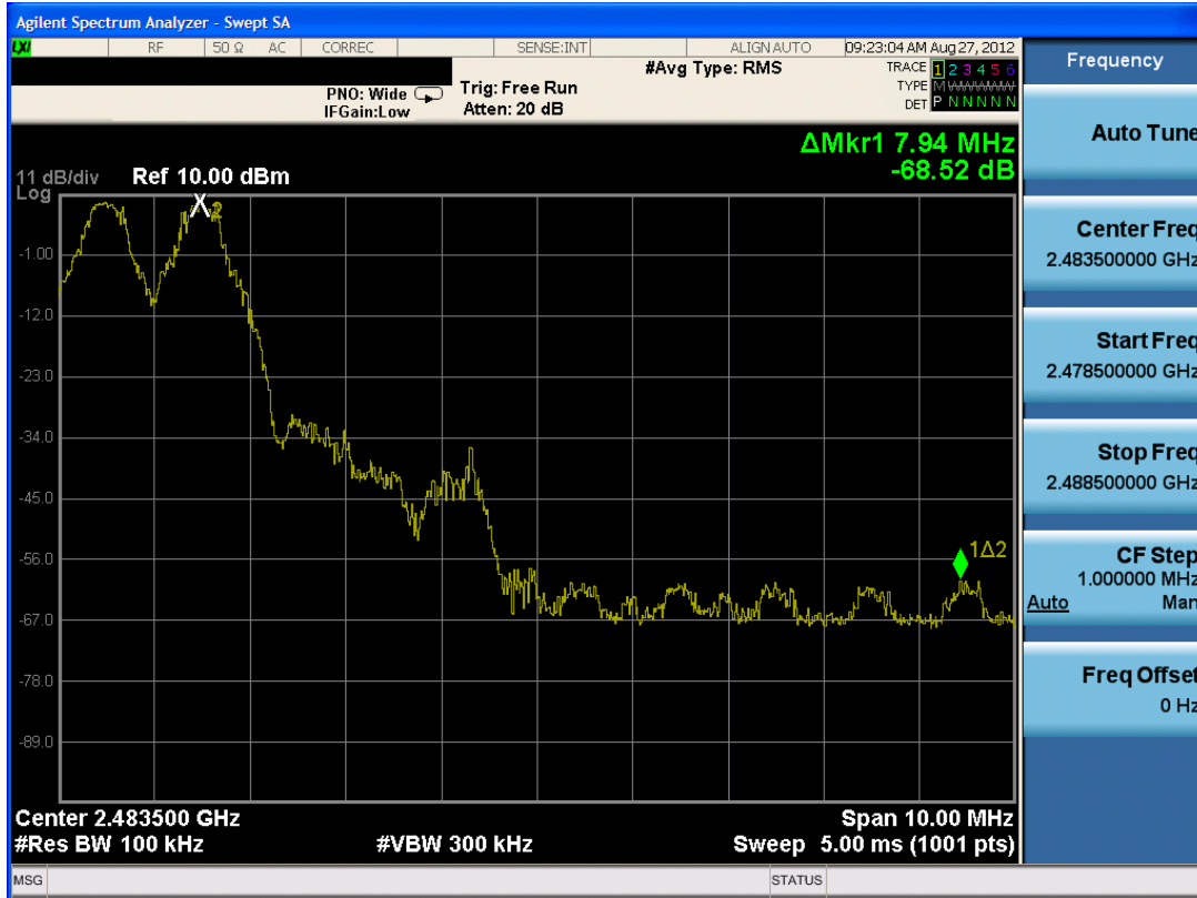
Plot 6-22. Band Edge Plot (Bluetooth with Hopping Enabled, 1Mbps)
