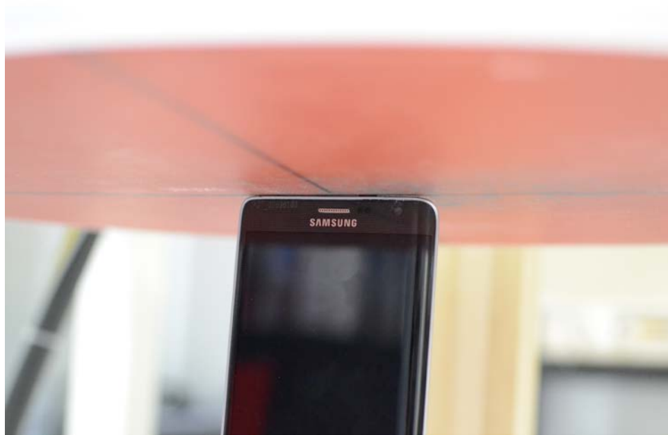
SAR Test Setup Photo 10 – Top Edge at 0.0 cm
