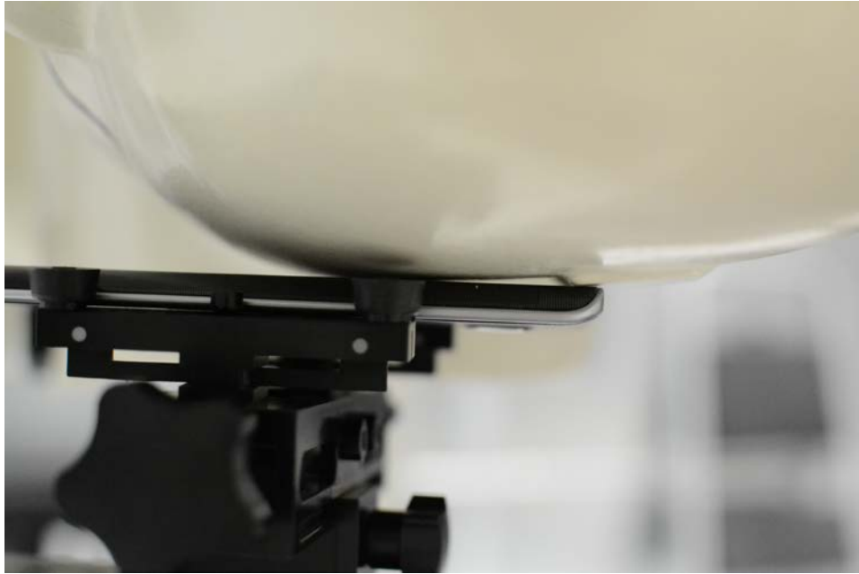
SAR Test Setup Photo 3 – Left Cheek
