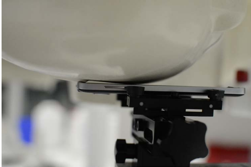
SAR Test Setup Photo 1 – Right Cheek
