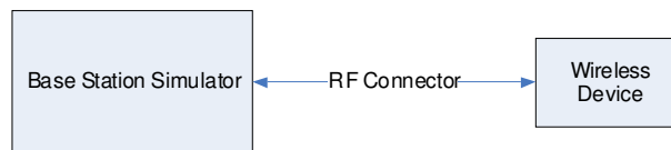
Figure 11-1 Power Measurement Setup
