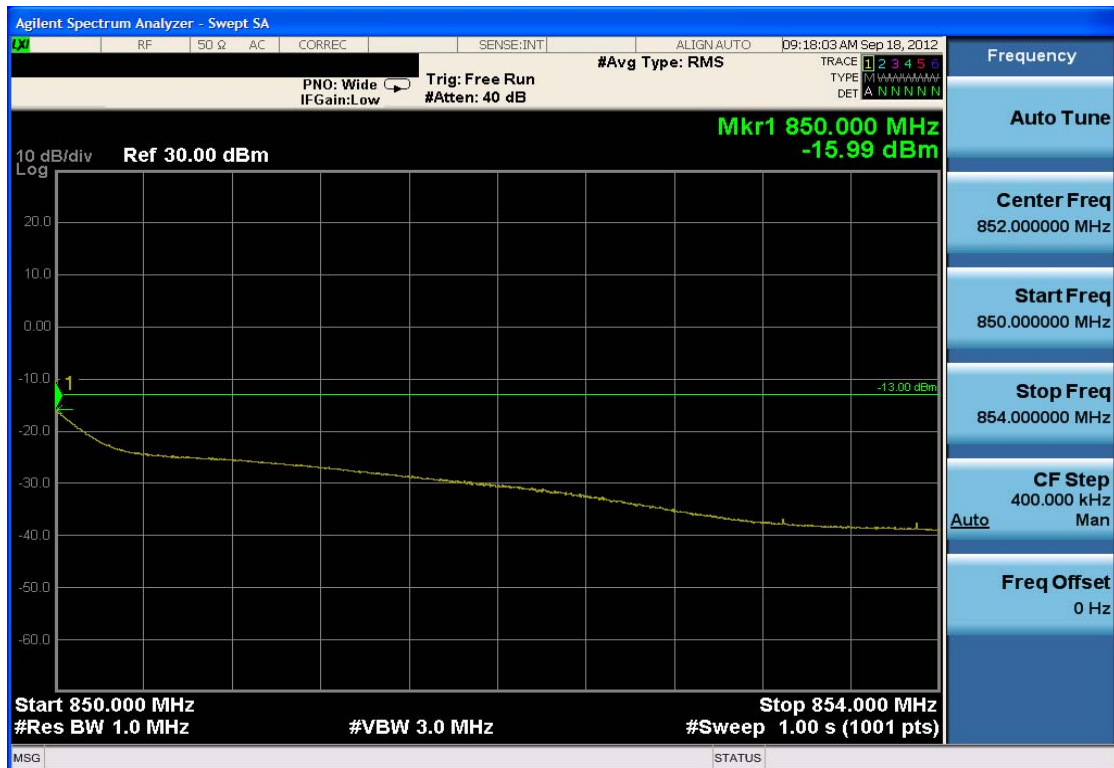
Plot 7-36. 4MHz Span Plot (Cellular WCDMA Mode – Ch. 4233)
