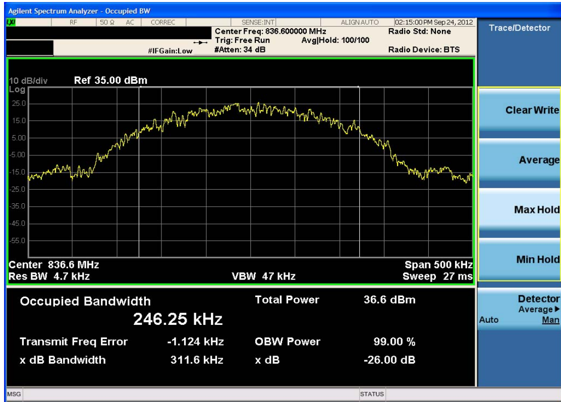
Plot 7-13. Occupied Bandwidth Plot (EDGE850 Mode – Ch. 190)
