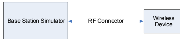
Figure 8-2 Power Measurement Setup
