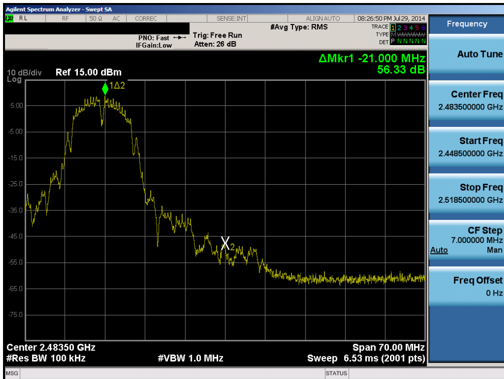
Plot 6-74. Band Edge Plot (802.11b – Ch. 11)
