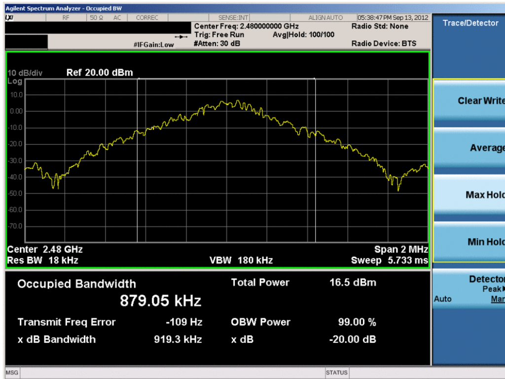
Plot 6-3. 20dB Bandwidth Plot (Bluetooth, 1Mbps – Ch. 78)
