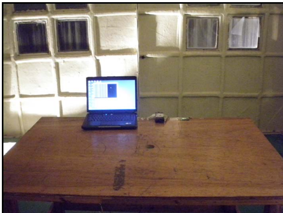
Photograph 2: Setup for Radiated Emissions
