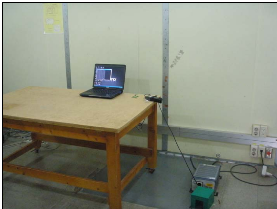
Photograph 1: Setup for Conducted Emissions
