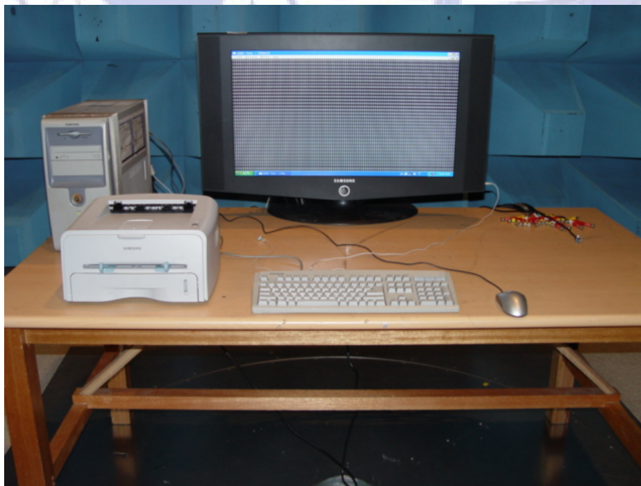
Picture 2. Radiated Emission (front view)
