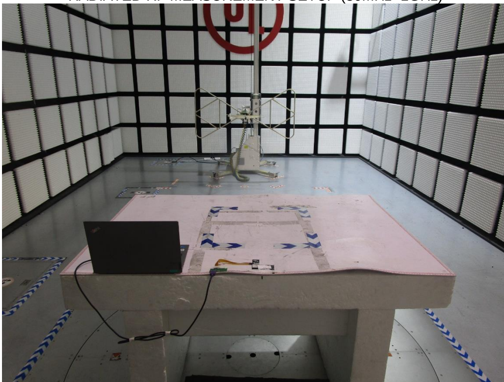
RADIATED RF MEASUREMENT SETUP (Below 30MHz)
