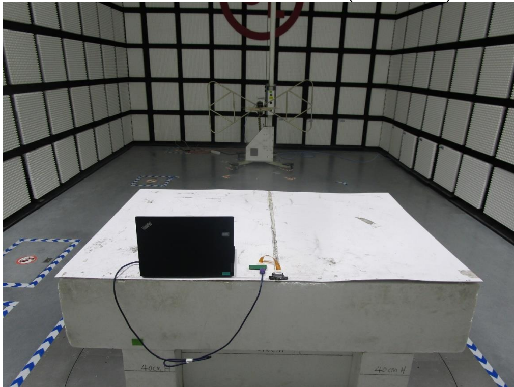
RADIATED RF MEASUREMENT SETUP (Below 30MHz)
