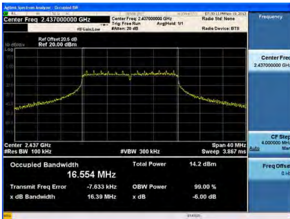
6dB Bandwidth plot (802.11g-CH 6)
