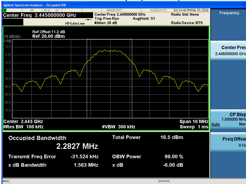
99% Bandwidth plot (Mid-CH 18)
