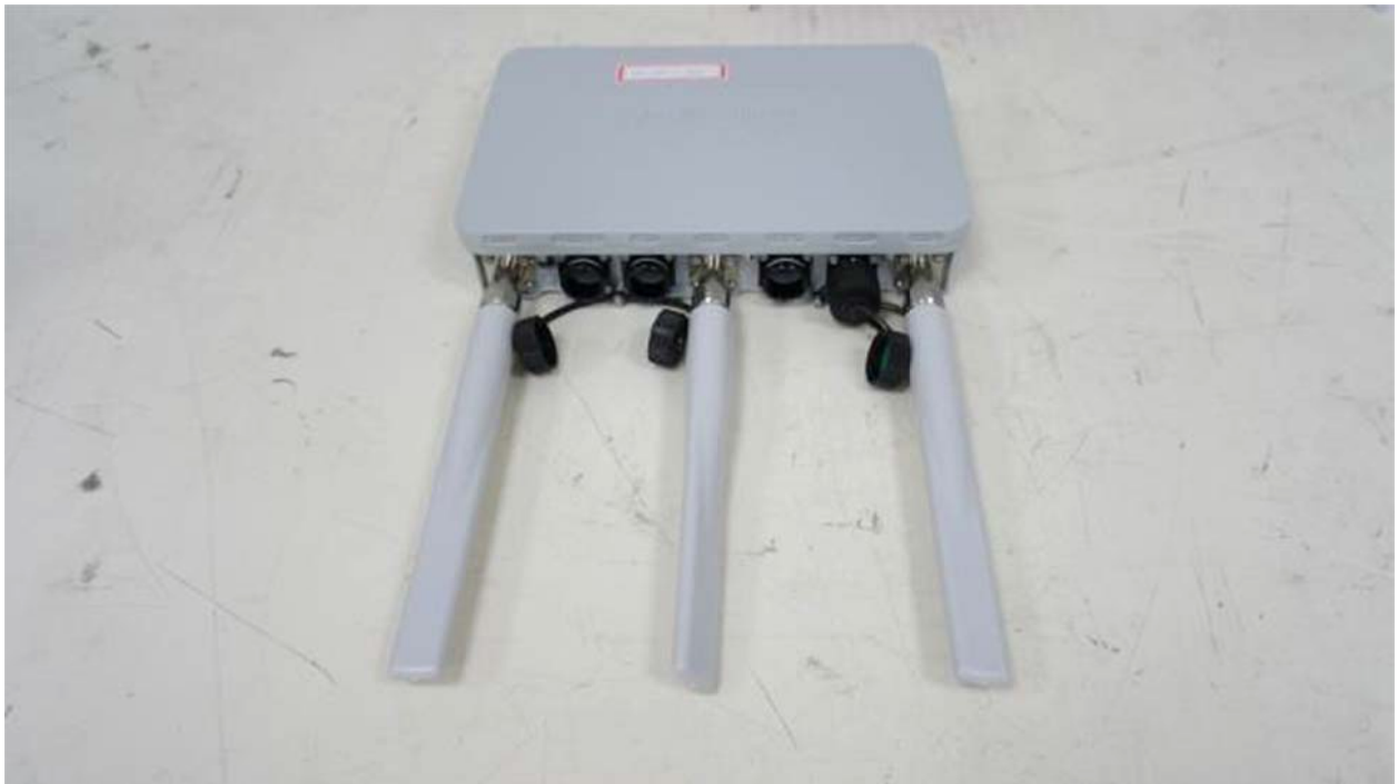
Front View (Dipole Antenna)
