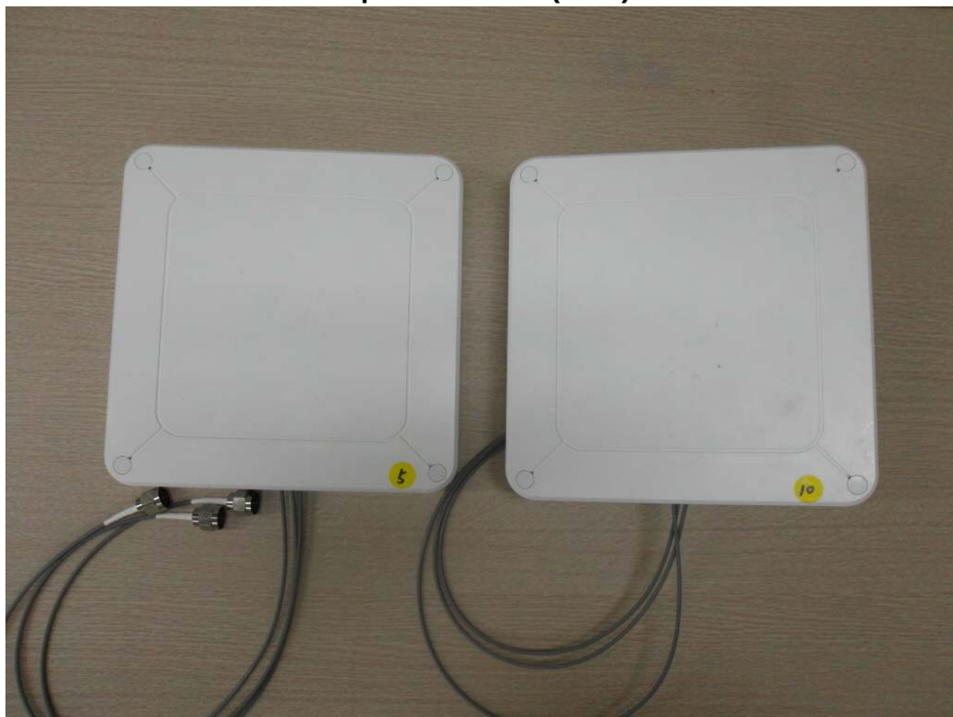
Patch Antenna # 1 (2 ea)
