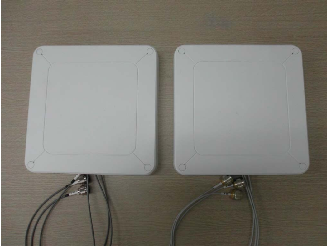
Patch Antenna# 2 (2 ea)
