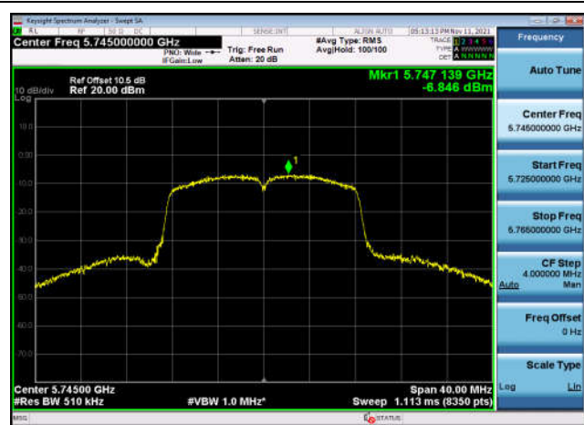
U-NII-3 Power spectral density-802.11 a(20MHz),5825MHz,Ant1
