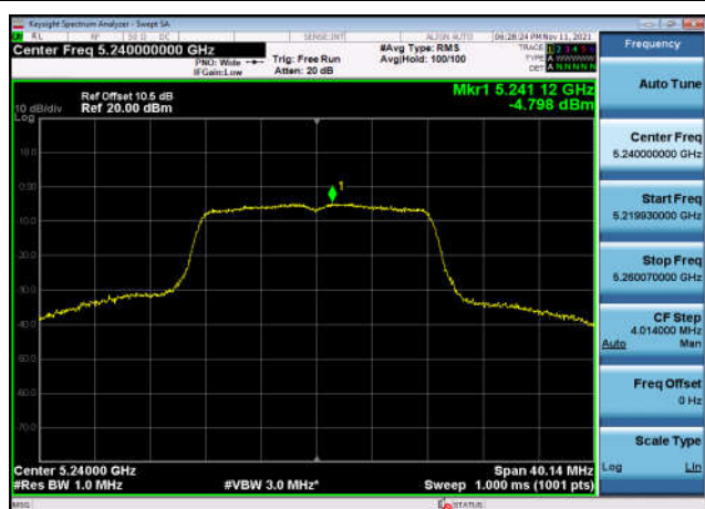
U-NII-1 Power spectral density-802.11 a(20MHz),5240MHz,Ant1
