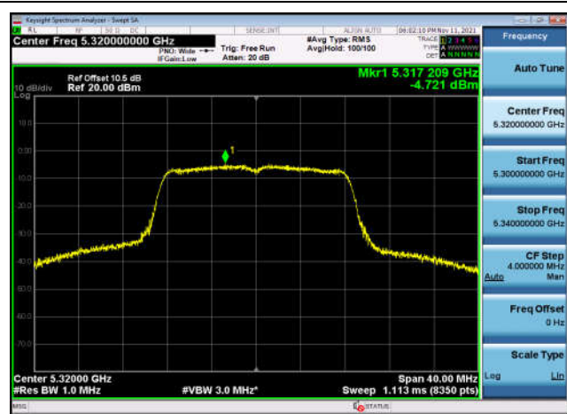
U-NII-2a Power spectral density-802.1 1a(20MHz),5320MHz,Ant1
