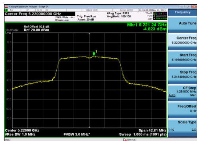
U-NII-1 Power spectral density-802.11 a(20MHz),5220MHz,Ant1
