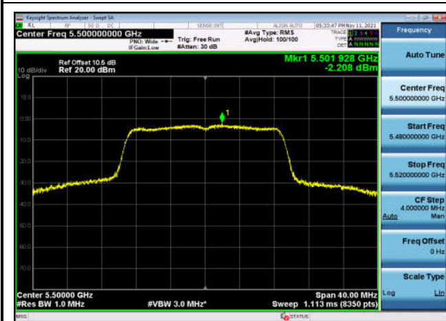
U-NII-2c Power spectral density-802.1 1n(20MHz),5700MHz,Ant1
