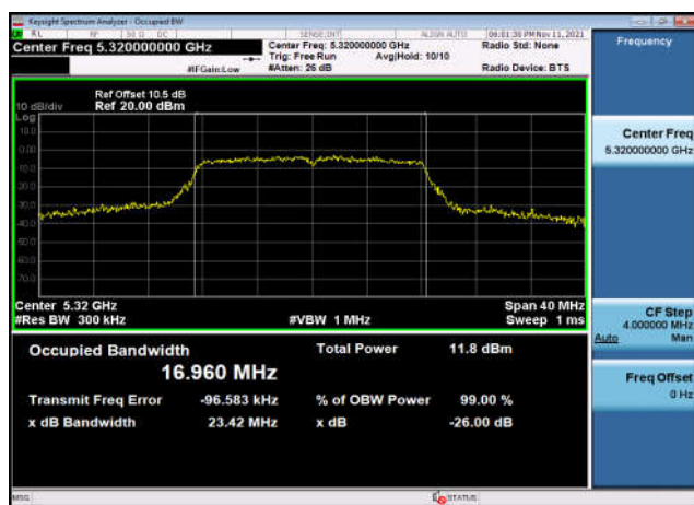
U-NII-2a 99% Bandwidth-802.11a(20MHz) ,5320MHz,Ant1
