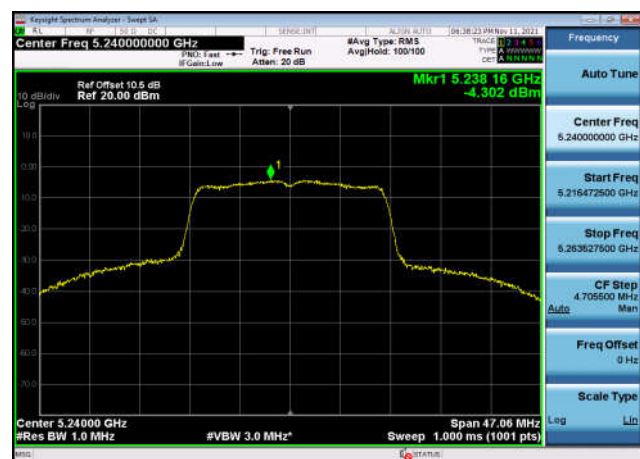
U-NII-1 Power spectral density-802.11 a(20MHz),5220MHz,Ant1
