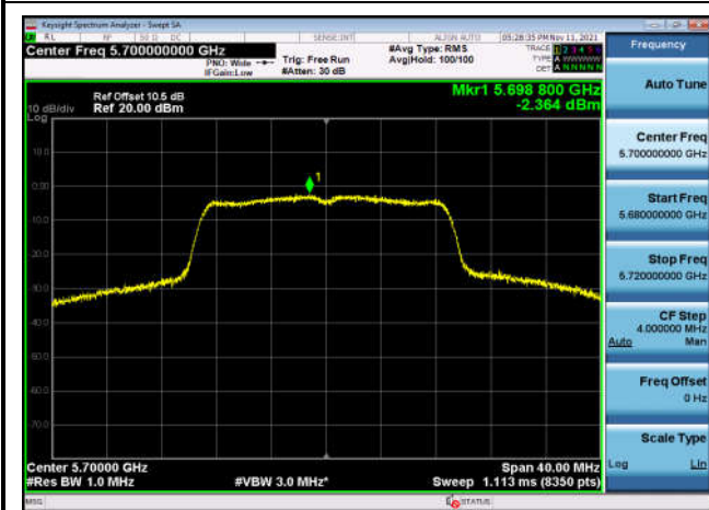
U-NII-2c Power spectral density-802.1 1a(20MHz),5600MHz,Ant1
