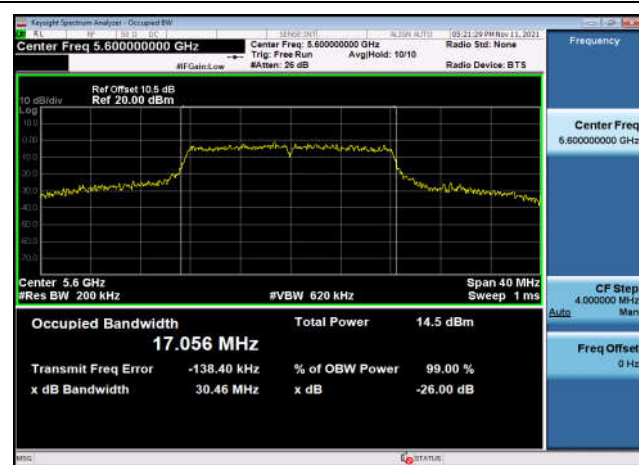
U-NII-2c 26dB Bandwidth-802.11a(20MHz ) ,5600MHz,Ant1
