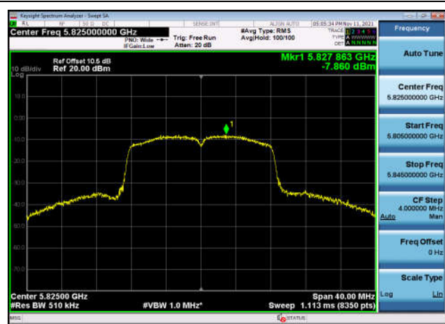
U-NII-3 Power spectral density-802.11 a(20MHz),5825MHz,Ant1
