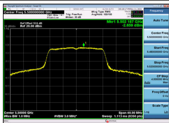
U-NII-2c Power spectral density-802.1 1a(20MHz),5700MHz,Ant1
