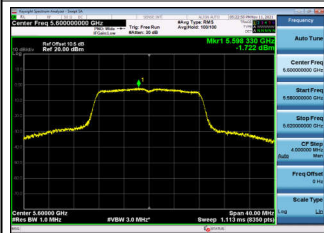
U-NII-2c Power spectral density-802.1 1a(20MHz),5600MHz,Ant1
