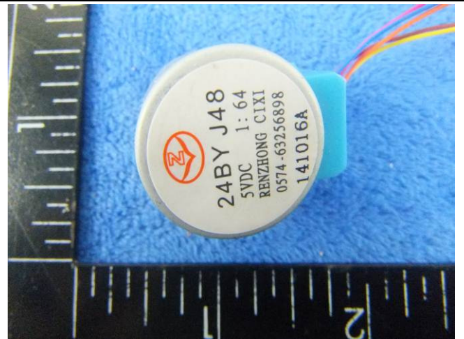
Motor - Front View
