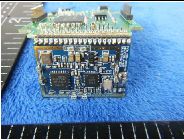
FHSS Board without shielding - Front View
