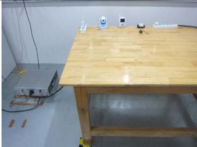
Conducted Emissions Test Setup – 433MHz Front View
