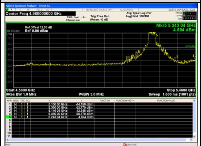
Out Of Band Emission IEEE 802.11ac_Channel 46_40MHz_Antenna 0
