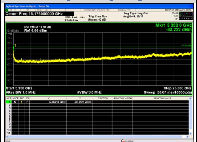
Spurious Emission:5350~25000.0 MHz IEEE 802.11ac_Channel 46_40MHz_Antenna 0
