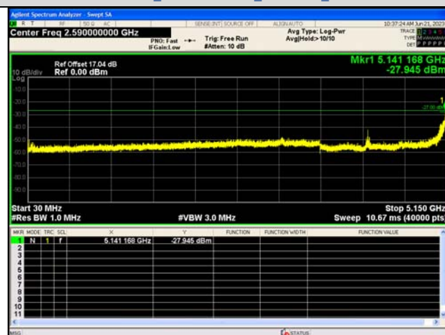
Spurious Emission:30.0~5150 MHz IEEE 802.11ac_Channel 46_40MHz_Antenna 0
