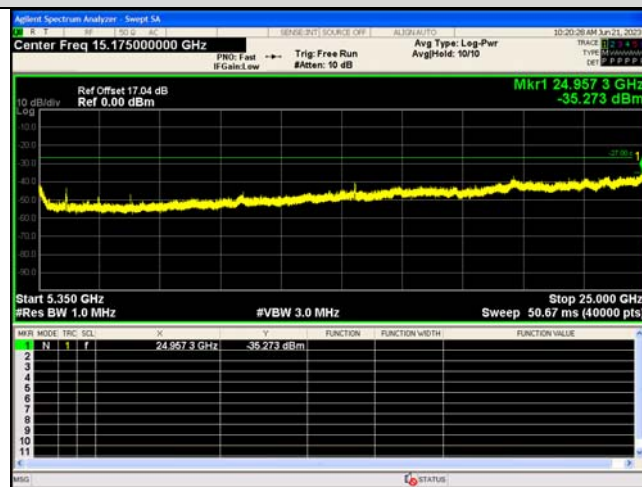
Spurious Emission:5350~25000.0 MHz IEEE 802.11ac_Channel 40_20MHz_Antenna 0
