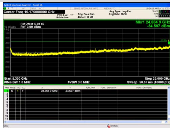
Spurious Emission:5350~25000.0 MHz IEEE 802.11ac_Channel 52_20MHz_Antenna 0
