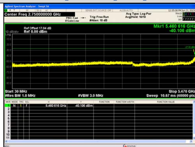
Spurious Emission:30.0~5470 MHz IEEE 802.11ac_Channel 118_40MHz_Antenna 0
