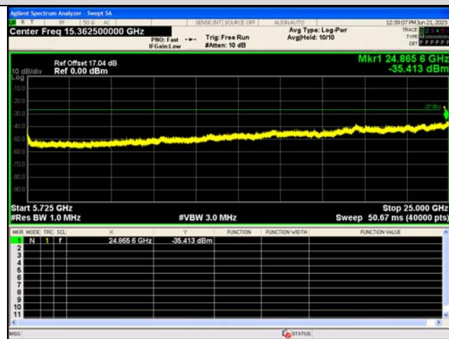
Spurious Emission:5725~25000.0 MHz IEEE 802.11ac_Channel 134_40MHz_Antenna 0
