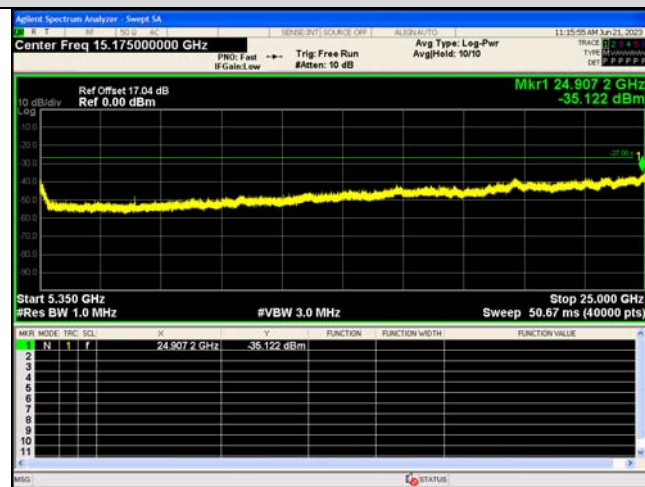
Spurious Emission:5350~25000.0 MHz IEEE 802.11n_Channel 54_40MHz_Antenna 0
