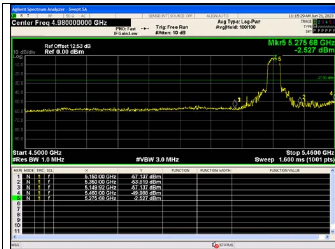
Out Of Band Emission IEEE 802.11n_Channel 54_40MHz_Antenna 0
