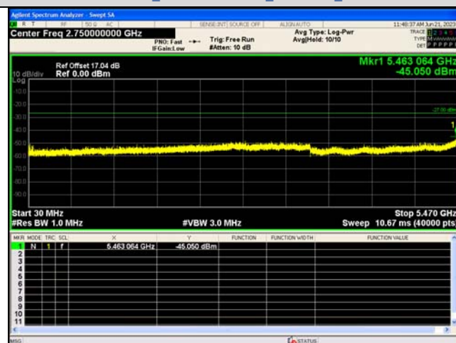
Spurious Emission:30.0~5470 MHz IEEE 802.11ac_Channel 140_20MHz_Antenna 0
