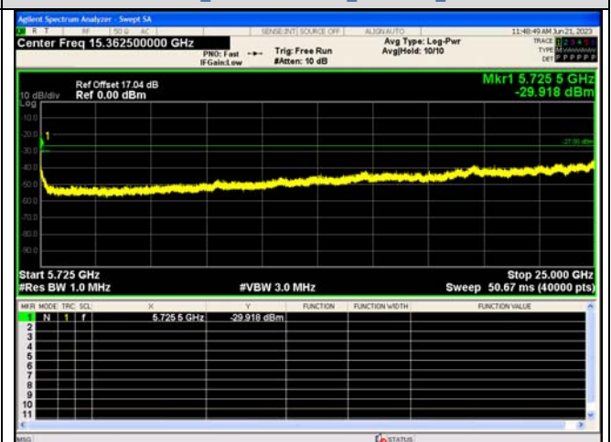
Spurious Emission:5725~25000.0 MHz IEEE 802.11ac_Channel 140_20MHz_Antenna 0
