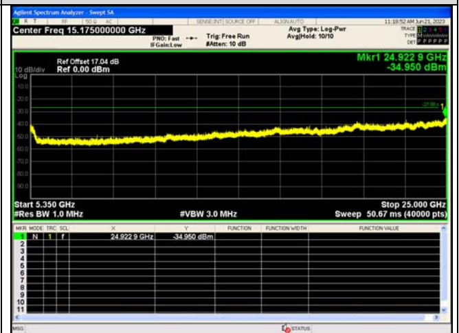
Spurious Emission:5350~25000.0 MHz IEEE 802.11n_Channel 62_40MHz_Antenna 0
