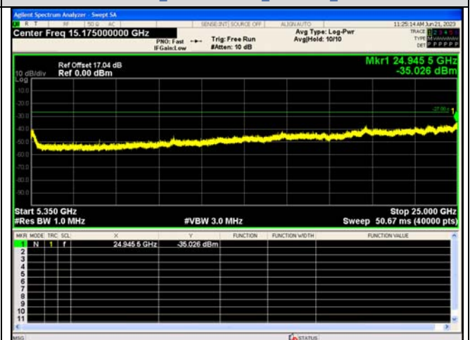
Spurious Emission:5350~25000.0 MHz IEEE 802.11ac_Channel 62_40MHz_Antenna 0
