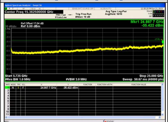
Spurious Emission:5725~25000.0 MHz IEEE 802.11ac_Channel 118_40MHz_Antenna 0
