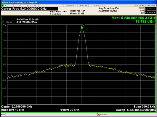
NT/NV_Antenna 0 IEEE 802.11ac Channel 48_20MHz
