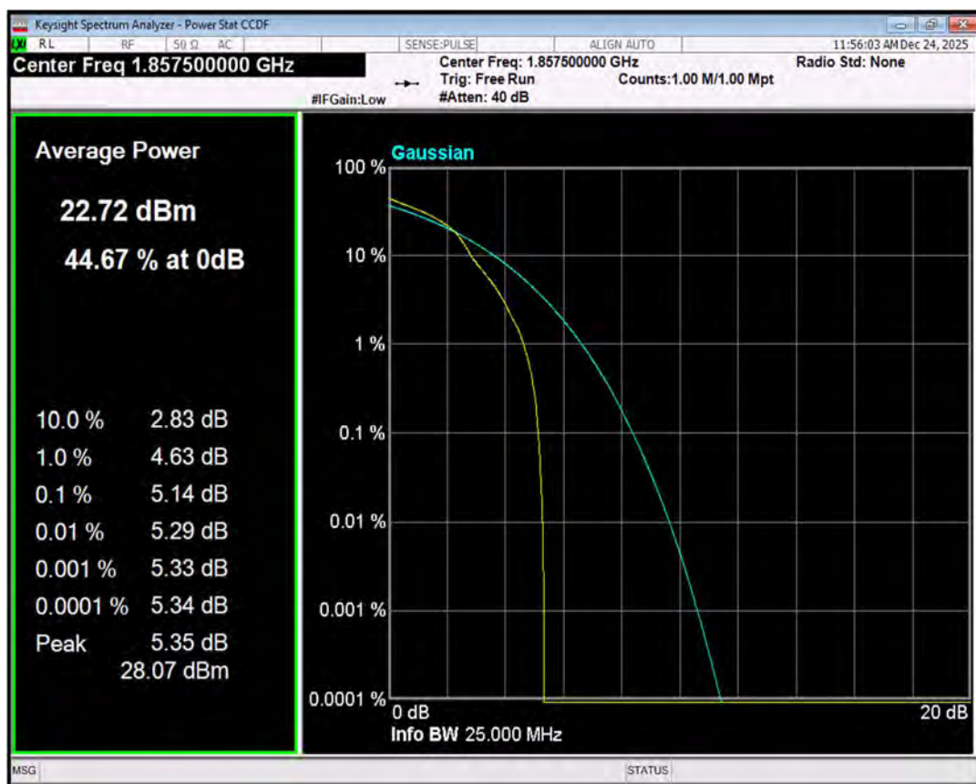
Band2 16QAM BW=15MHz Channel=18900 RB Size=1 Position=#0
