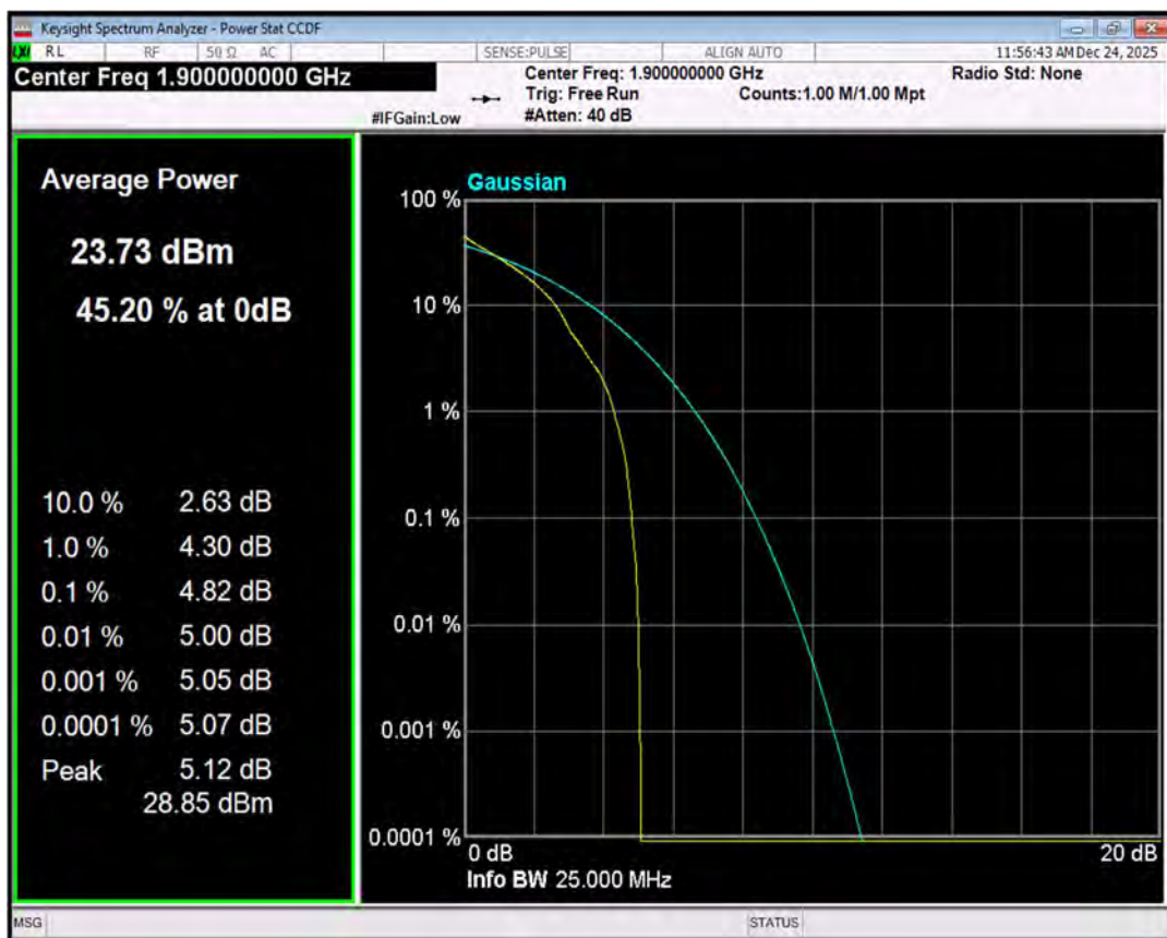
Band2 QPSK BW=3MHz Channel=18615 RB Size=1 Position=#0
