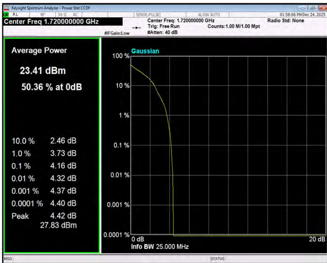
Band66 QPSK BW=20MHz Channel=132322 RB Size=1 Position=#0
