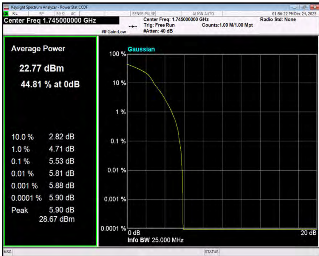
Band66 16QAM BW=3MHz Channel=132657 RB Size=1 Position=#0
