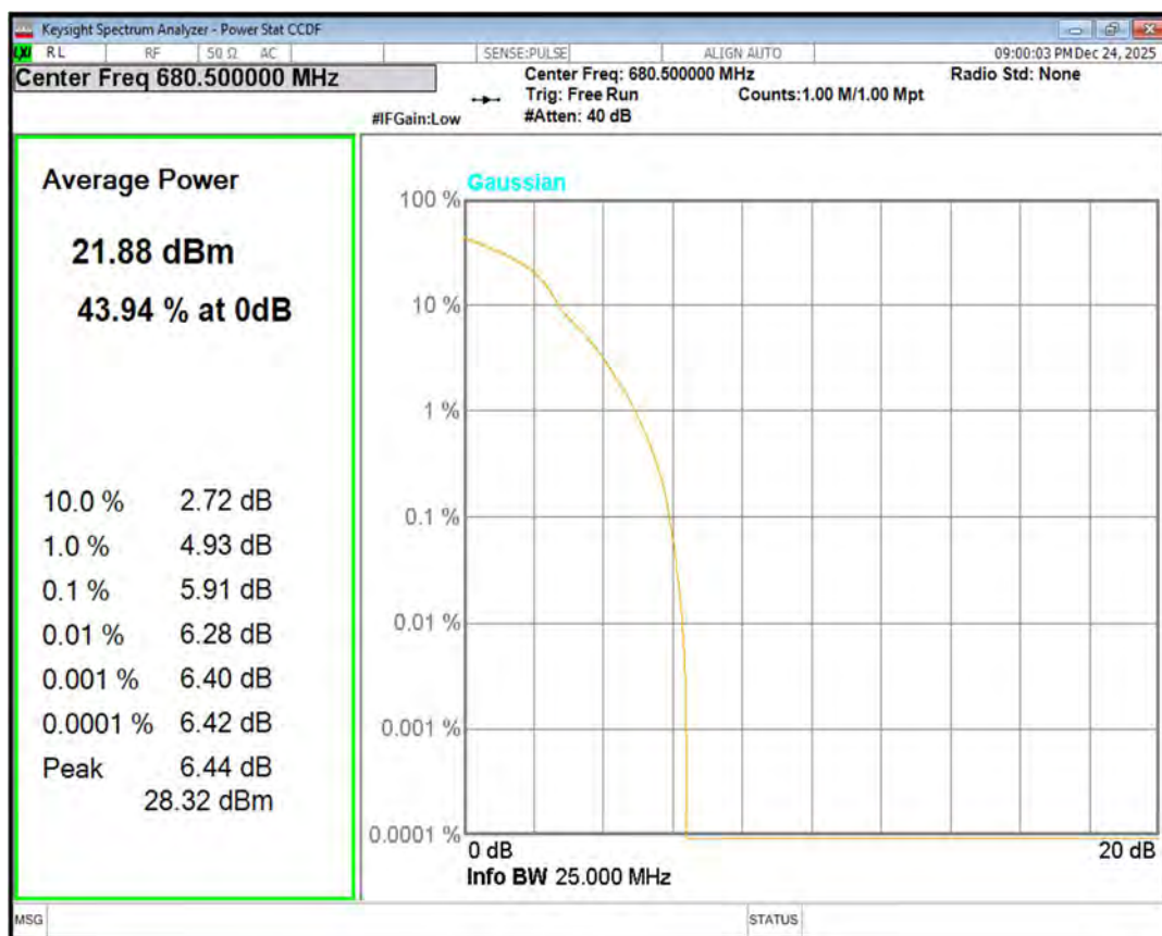
Band71 16QAM BW=5MHz Channel=133447 RB Size=1 Position=#0
