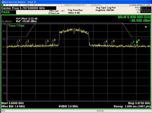
Out Of Band Emission IEEE 802.11ac_Channel 155_80MHz_Antenna 0
