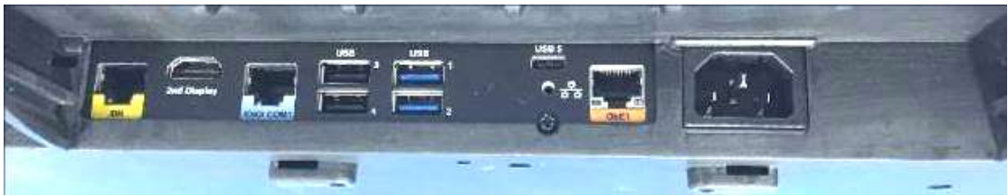
Figure 1-3: MICROS Express Station 4 I/O View
