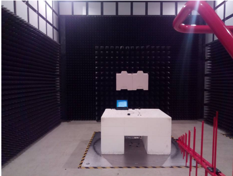
Radiated Emissions – Front View (Below 1 GHz)
