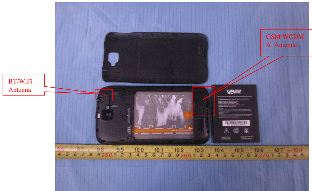
EUT – Cover off View 1
