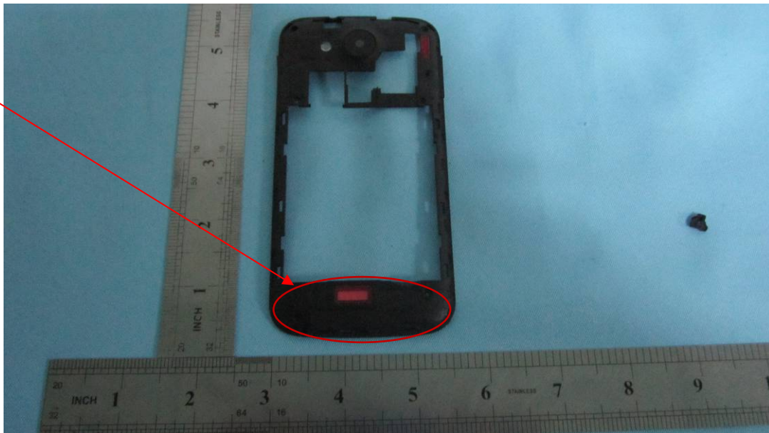
GSM / PCS/ UMTS Antenna View
