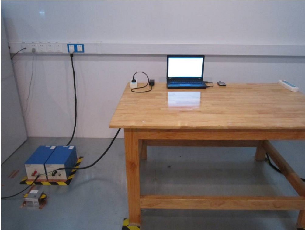
Conducted Emissions Test Setup Front View
