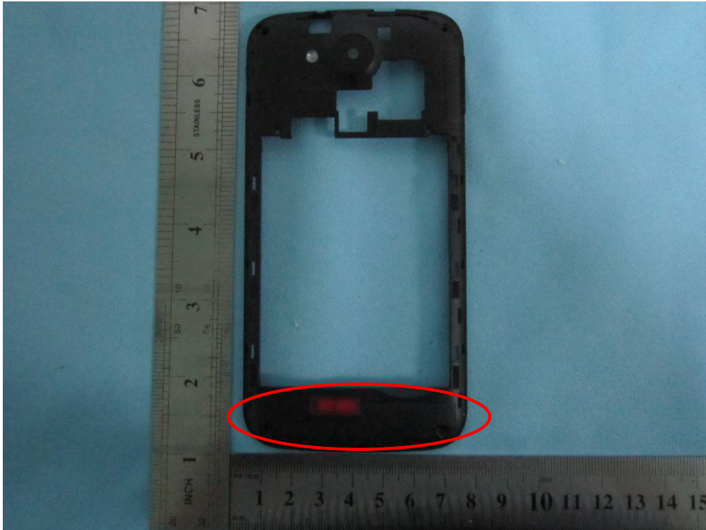
GSM / PCS/ UMTS Antenna View
