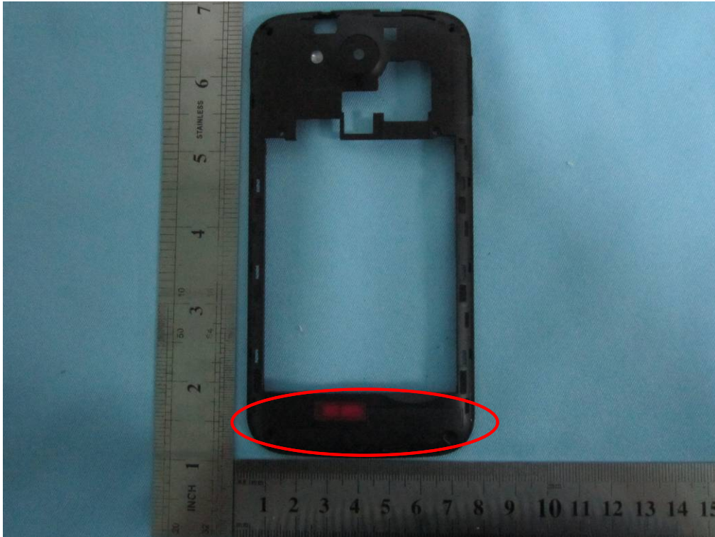
GSM / PCS/ UMTS Antenna View
