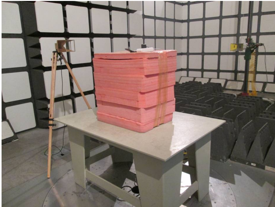
Radiated Emissions View (Above 1 GHz)
