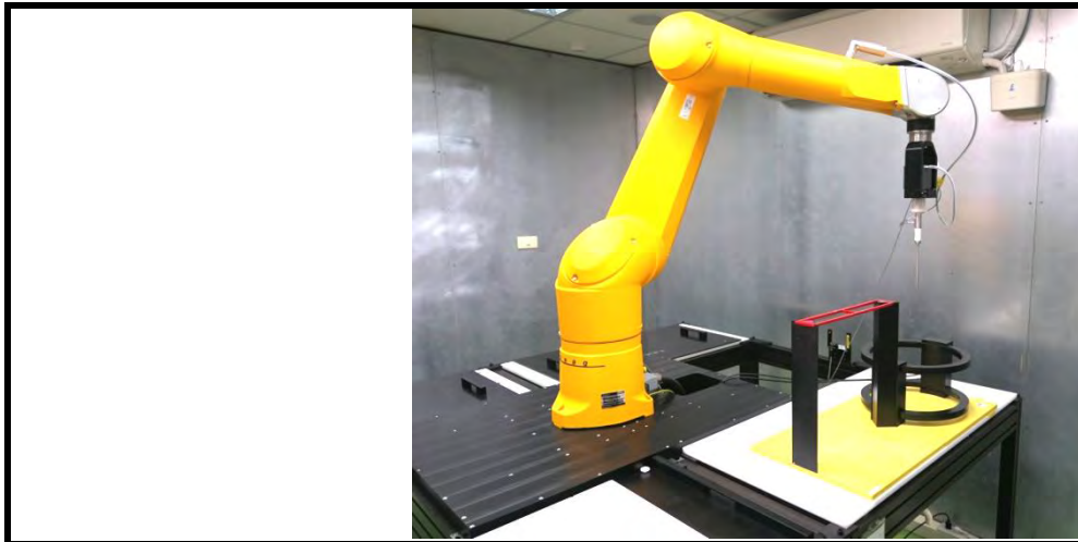
Fig-3.3 DASY5 Measurement System
