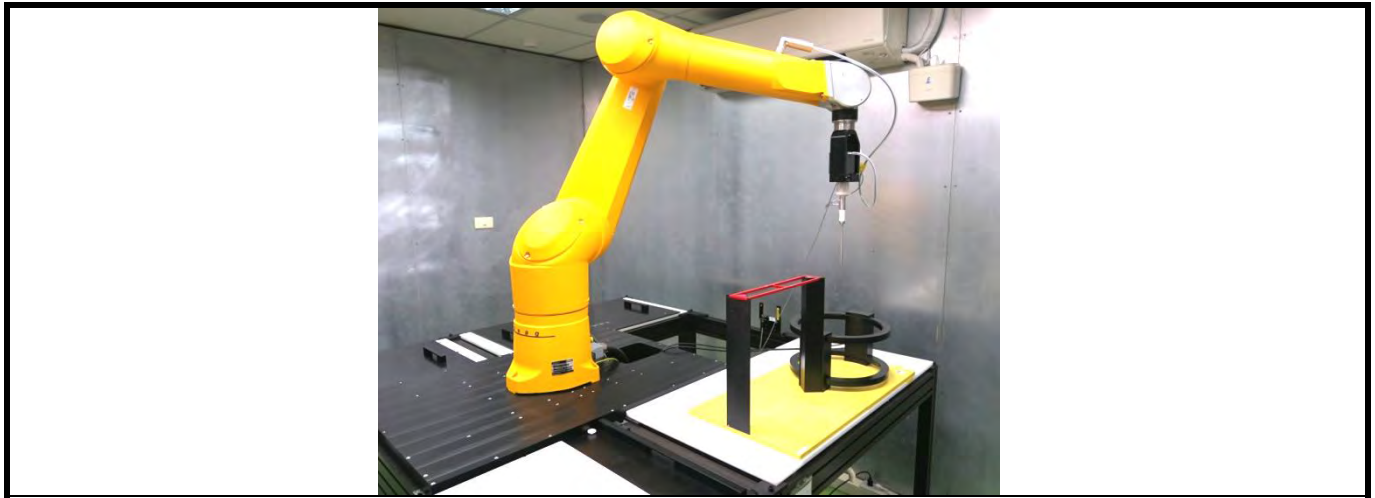
Fig-3.3 DASY52 Measurement System
