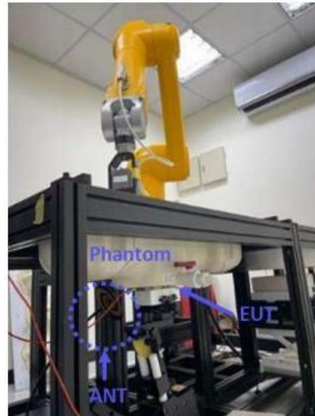
Figure 5-3 The other view of DASY6 TA-SAR test environment
