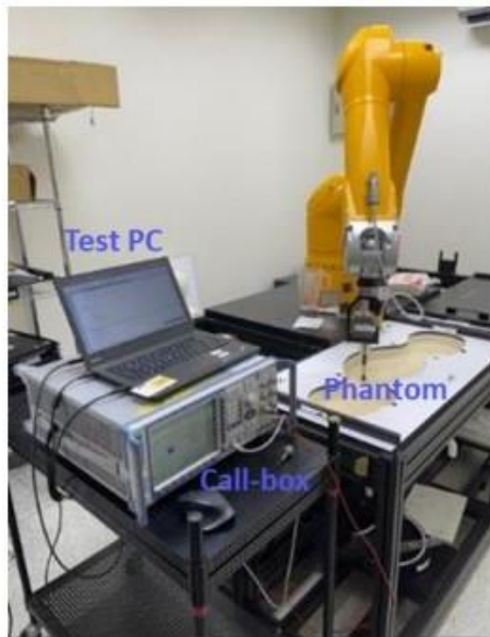
Figure 5-2 DASY6 TA-SAR test environment with call box and PC
