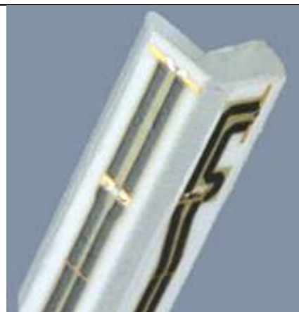
Fig 5.2 Photo of E-field Probe
